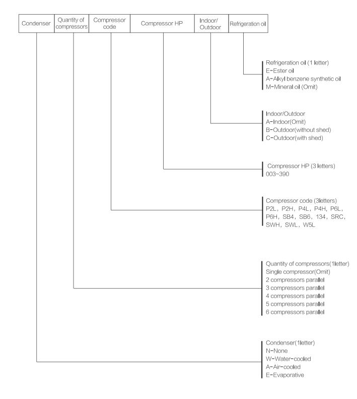
Note: N2SW3L080A, means 2sets SW3L8000(80HP) semi-hermetic compressors installed in one package without condenser, indoor-type 2compressors parallel package with alkyl benzene synthetic oil.
