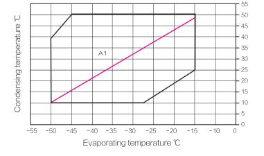
50Hz full load running 10K suction superheat A1⊠=oil cooler is required
