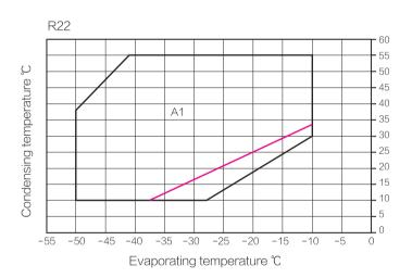
50Hz full load running 10K suction superheat A1⊠=oil cooler is required
